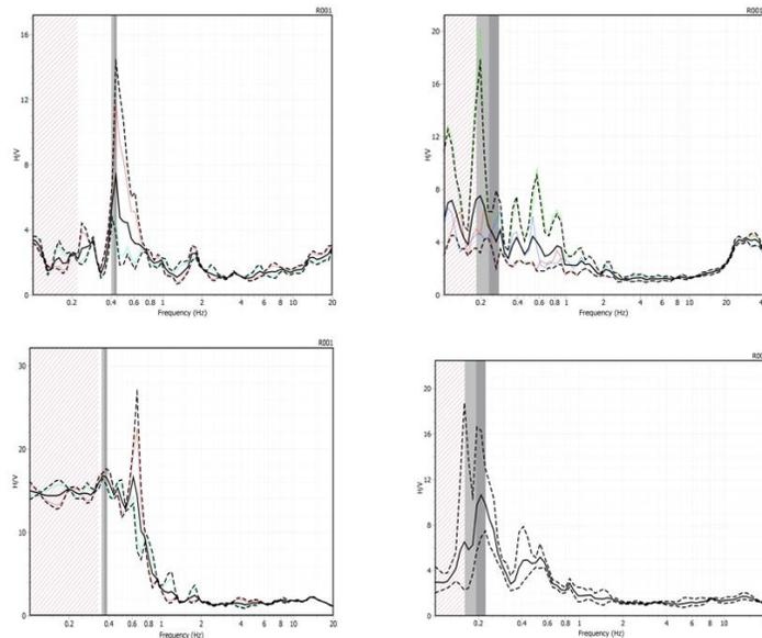
Fig (5). Samples of HVSR curves with fundamental frequency ranging between 0.2 and 0.45Hz
