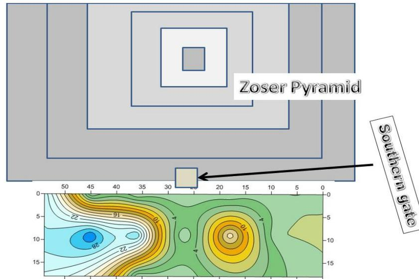
Fig. (7). Map distribution of fundamental frequencies at the fifteen sites in front of the southern edge of Zoser pyramid. Low fundamental frequency area is observed adjacent to the southern gate of the pyramid.
