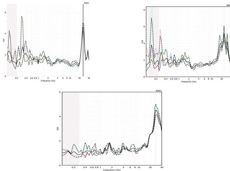
Fig. (6). Samples of HVSR curves showing high fundamental frequency that reach 32 Hz.
