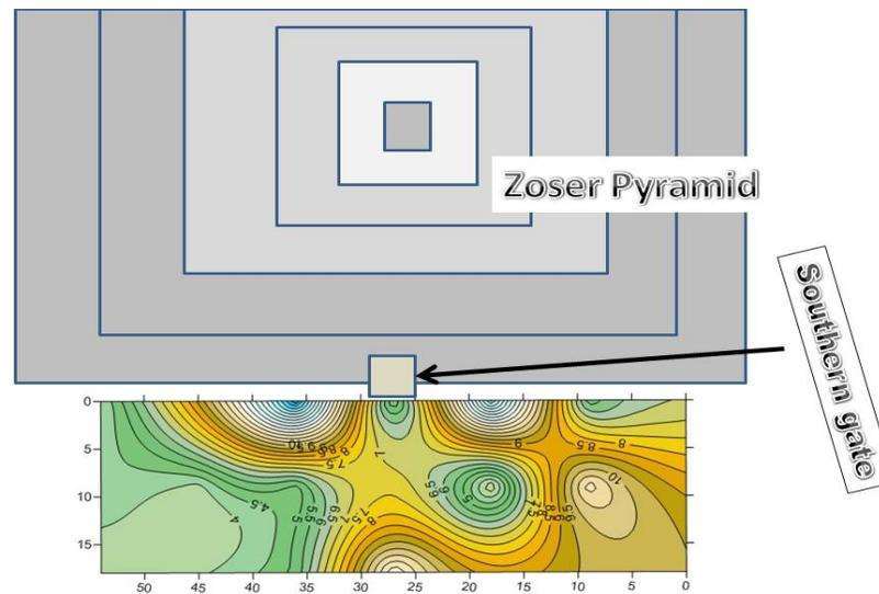
Fig. 8. Map distribution of Peak amplitudes of the HVSR curve. Again lower values is observable adjacent to the southern gate of the pyramid.
