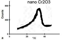
Fig. 3. XRD analysis of Cr<sub>2</sub>O<sub>3</sub> nanoparticles.
