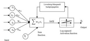
Fig. 4. Architecture of applied neural network.
