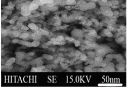
Fig. 2. SEM micrograph of Cr<sub>2</sub>O<sub>3</sub> nanoparticles.
