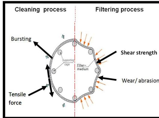
**Figure (2)** Mechanical Stresses and forces during filtering and cleaning in pulse-jet system
