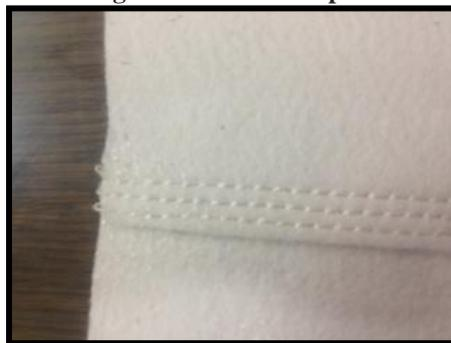
Figure (7): Three lines sewn filter bag
