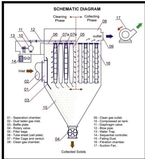
**Figure (1)** schematic diagram of a pulse-jet cleaned bag house and cleaning cycles
