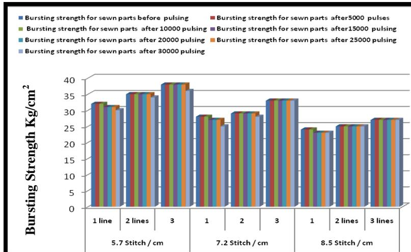
Figure (13) Bursting Strength (Sewing A)
