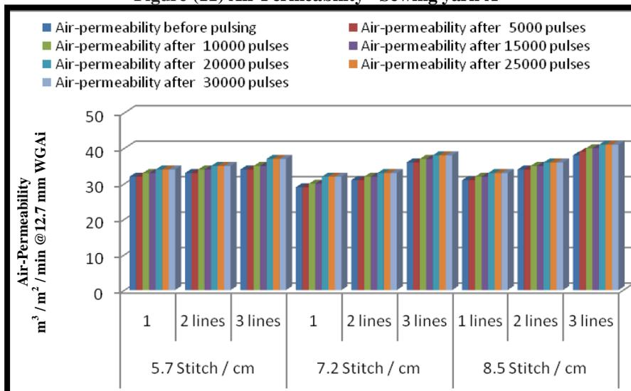
Figure (12) Air Permeability "Sewing yarn B"
