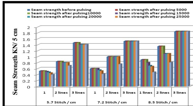
**Figure (16) Seam strength (Sewing yarn B)**
