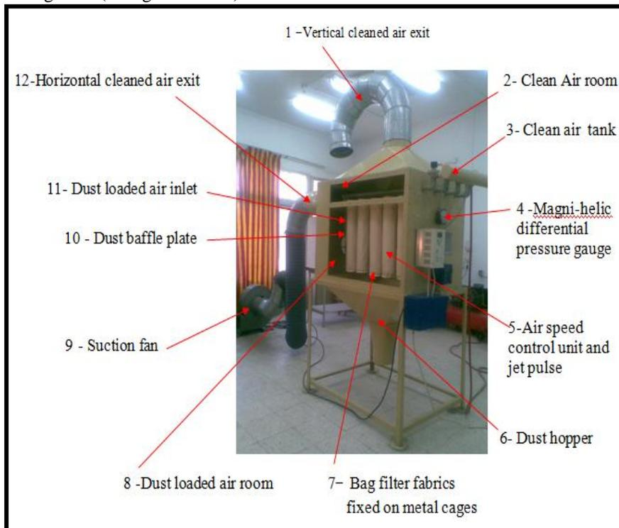
Figure (10): Pilot scale bag filter unit
