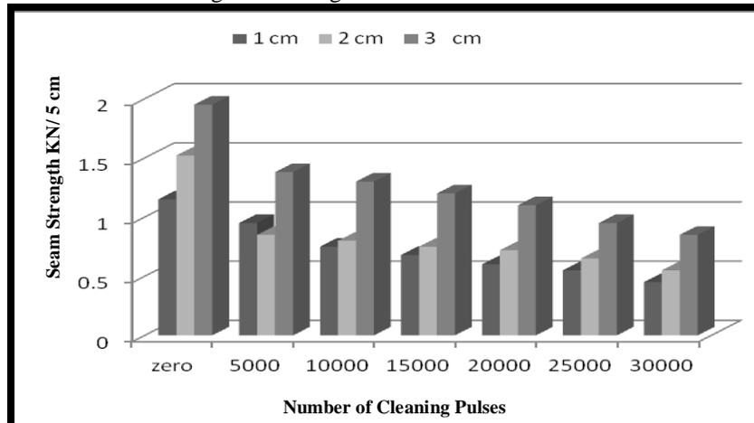
Figure (19) Welding Tensile Strength
