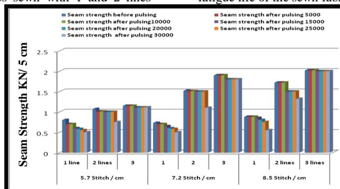
Figure (15) Seam strength (Sewing yarn A)
