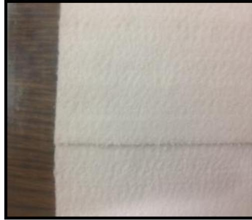
Figure (9): Welded filter fabric
