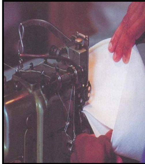
Figure 5 Anti-collapse rings into filter Bags using lock stitching
