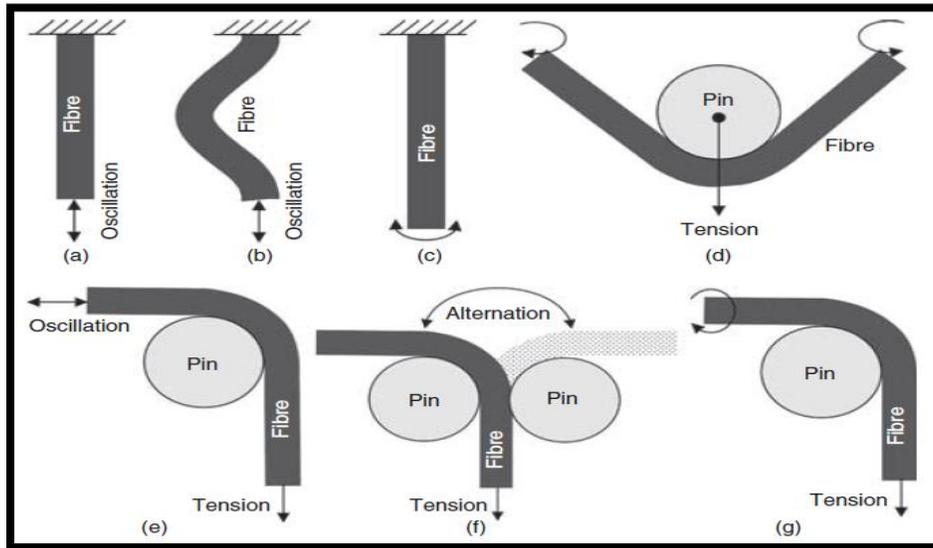
**Figure (3)** Examples of fiber fatigue simulation
