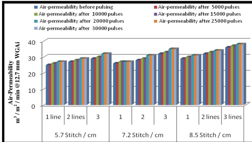
Figure (11) Air Permeability "Sewing yarn A"
