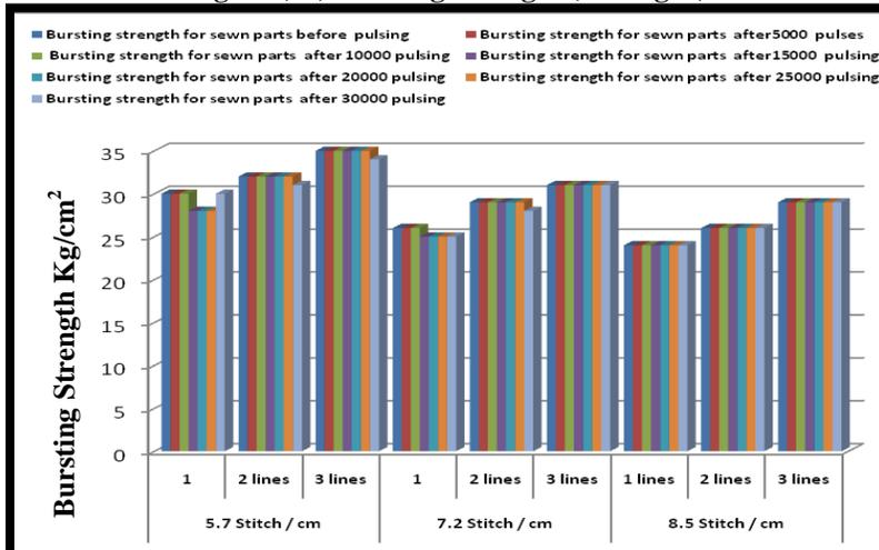
Figure (14) Bursting Strength (Sewing B)
