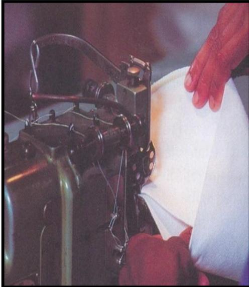
Figure 4 Discs (metal rings) are sewn to the filter bag with an over lock stitch
