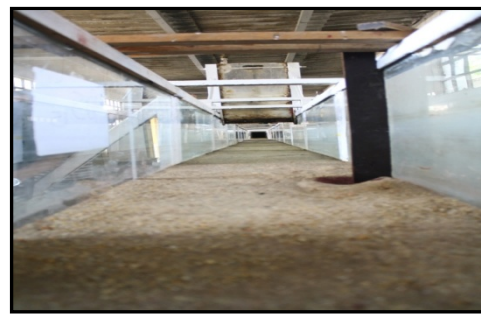
Figure1: General View of the Used Flume
