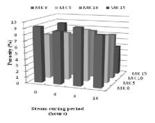
Figure 1. Porosity at different metakaolin replacement levels and steam curing period at 1Day
