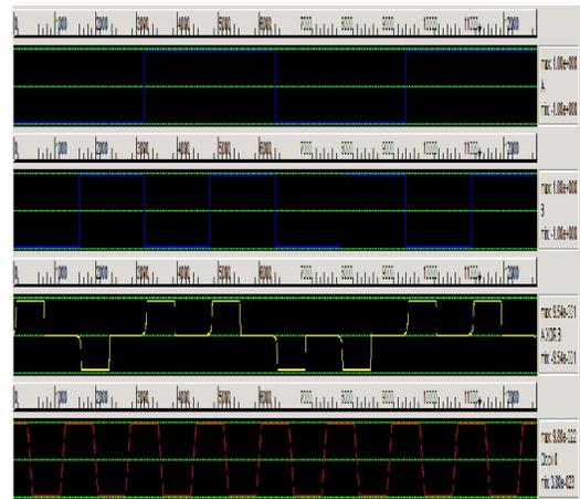
Figure 14. Results of Simulation of the Suggested XOR gate
