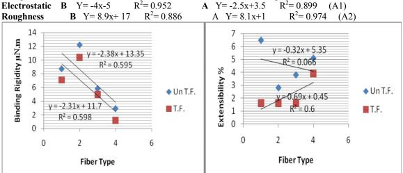
Fig.(3):Regression Line between Fiber Type& Bending Rigidity before and after Treatment **Bending Rigidity B** Y= -2.38x+13.35 R<sup>2</sup>= 0.595 Fig.(4):Regression Line between Fiber Type& Extensibility before and after Treatment A = -2.31x+11.7 R<sup>2</sup>= 0.598 (A3)
