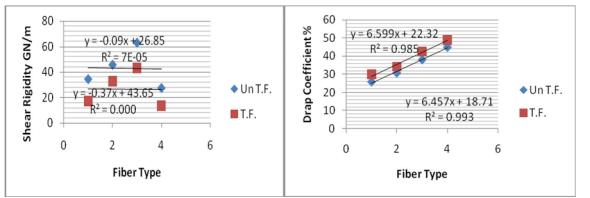
Fig. (7): Regression Line between Fiber Type & ShearFig. (8): Regression Line between Fiber Type & DrapeRigidity before and after TreatmentCoefficient before and after Treatment
