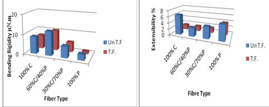
Fig. (13): The Relation between Fiber Type& BendingFig. (14): The Relation between Fiber Type &Rigidity before and after TreatmentExtensibility before and after Treatment
