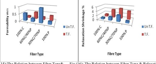
Fig. (15): The Relation between Fiber Type& Formability before and after Treatment
