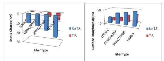
Fig. (11): The Relation between Fiber Type& ElectrostaticFig. (12): The Relation between Fiber Type & Chargesbefore and after TreatmentSurface Roughness before and after Treatment
