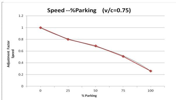
**Figure 3.** Effect coefficient of On-street park on average flow velocity in second-grade Main Street with trade usage
