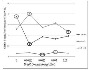
Figure 9. Effect of N-ZnO on Different Surfactants Static-Foam-Performance.
