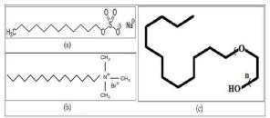
**Figure 1.** Schematic of (a): SDS, (b): CTAB, (c): LAE-7 Structures.
