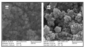
Figure 2. (a): SEM image of NS, (b): SEM image of N-ZnO.
