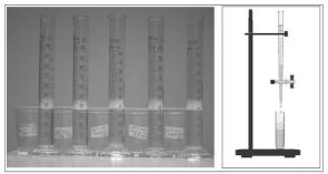
Figure 4. Static Foam Test Facilities.
