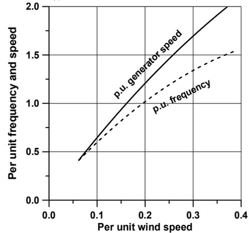
Fig. 6: Generator speed and frequency versus wind speed.
