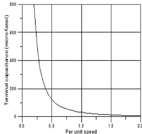
Fig. 5: Terminal capacitance versus per unit speed.
