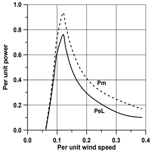
Fig. 9: Electrical and mechanical power versus wind speed.
