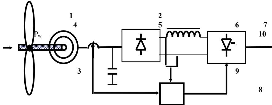
Fig. 1: Single line diagram of a wind energy driven SEIG connected to an infinite bus bar using a static power conditioner.
