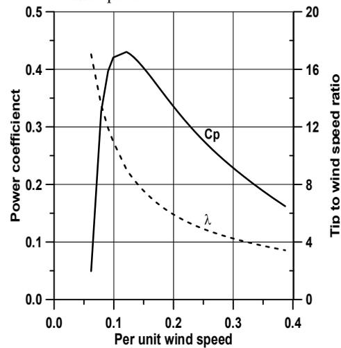
Fig. 7: Power coefficient and tip to wind speed ratio versus wind speed
