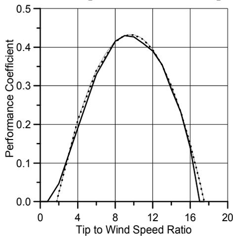
Fig. 4: Wind turbine performance curve, - - - - curve fitting approximation.
