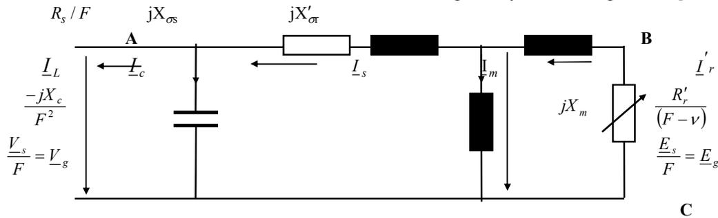
Fig. 3: Per phase steady state equivalent circuit of SEIG at load.
