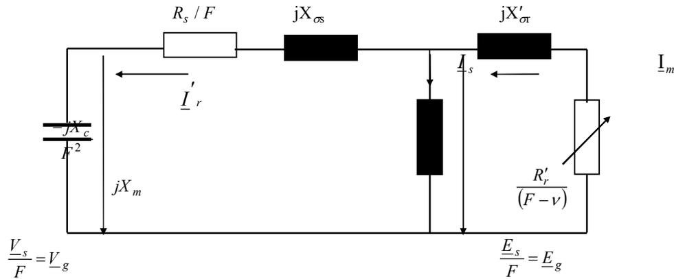
Fig. 2: Per phase steady state equivalent circuit of SEIG at no load.
