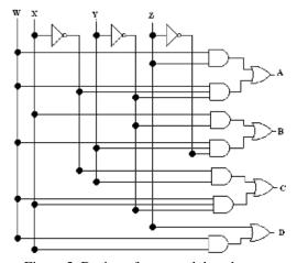
Figure 3. Design of proposed decoder
