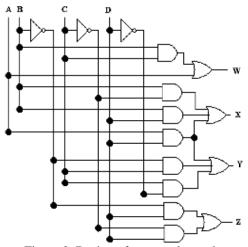
Figure 2. Design of proposed encoder
