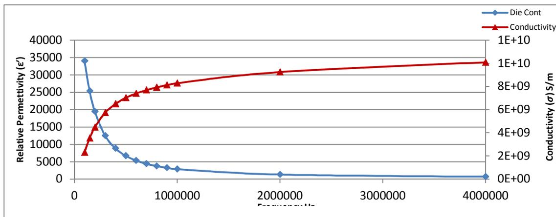
Figure-11: The variations of the relative permeability  $\epsilon'$  and electric conductivity  $\sigma$  as function of frequency in the range 0.1-10MHz for bacterial suspension exposed to 0.5 Hz PEF.
