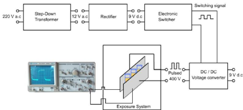
Figure-1: Schematic illustration of the experimental design used for exposure.
