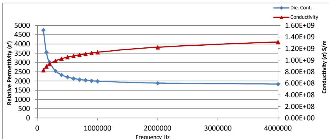
**Figuer-12:** The variations of the relative permeability  $\epsilon'$  and electric conductivity  $\sigma$  as function of frequency in the range 0.1-10MHz for bacterial suspension exposed to 0.7 Hz PEF.
