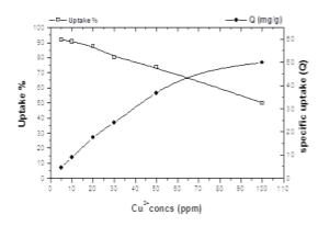
Fig. (3): Copper removal at different  $Cu^{2+}$  ions concentrations
