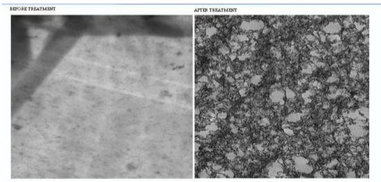
Fig. (12): TEM of Ca-alginate sorbent before and after copper sorption
