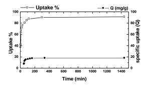
Fig. (7): Effect of Contact times on copper sorption
