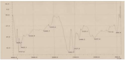
Fig. (9): FT-IR spectrum for Ca-alginate beads before treatment
