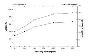
Fig. (8): Effect of stirring strength on copper sorption
