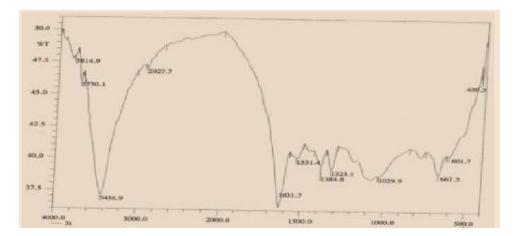
Fig. (10): FT-IR spectrum for Ca-alginate beads after treatment
