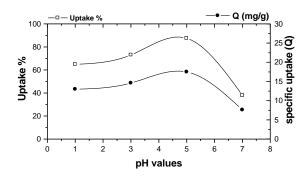
Fig. (2): Effect of solution pH on copper ion sorption
