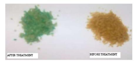
Fig. (11): Ca-alginate beads before & after treatment process
