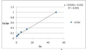
Fig. (4): Langmuir's isotherm for Cu<sup>2+</sup> removal by Ca-alginate beads
