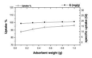
Fig. (6): Effect of adsorbent weights on copper sorption
