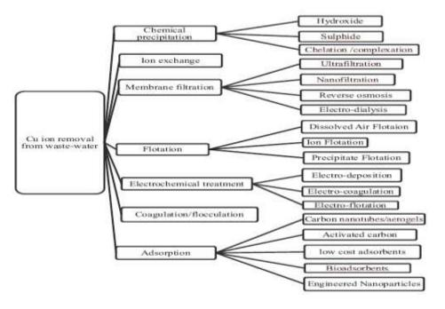
Fig. (1): Available treatment technologies for copper ion removal from wastewater
