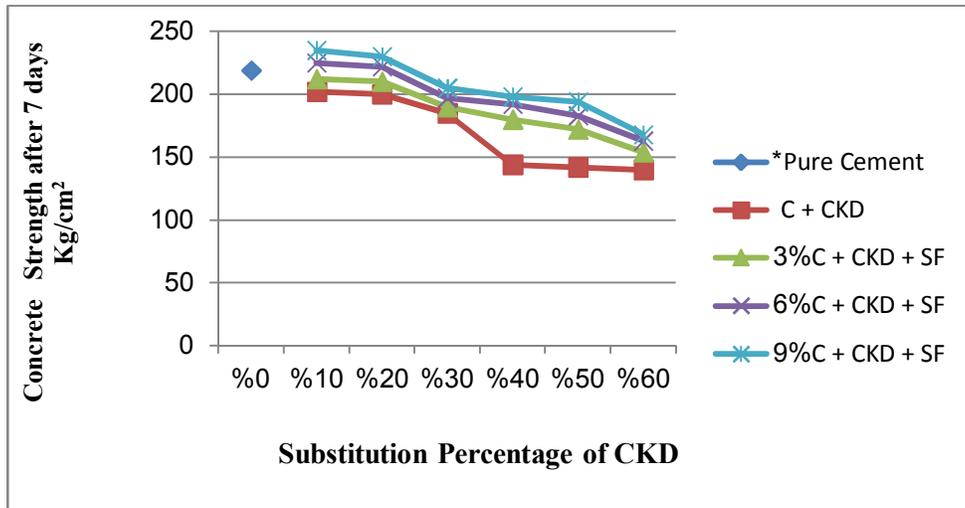
Fig(2) Concrete strength 7 days Versus Substitution percentage of CKD
