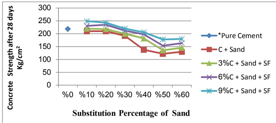
Fig(4) Concrete strength 28 days Versus Substitution percentage of Sand
