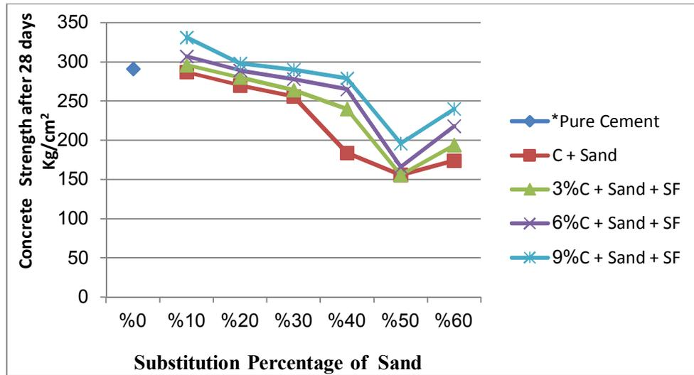
Fig(5) Concrete strength 28 days Versus Substitution percentage of Sand
