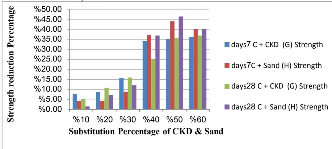
Fig (6)Percentage of Strength reduction for substitution percentage
