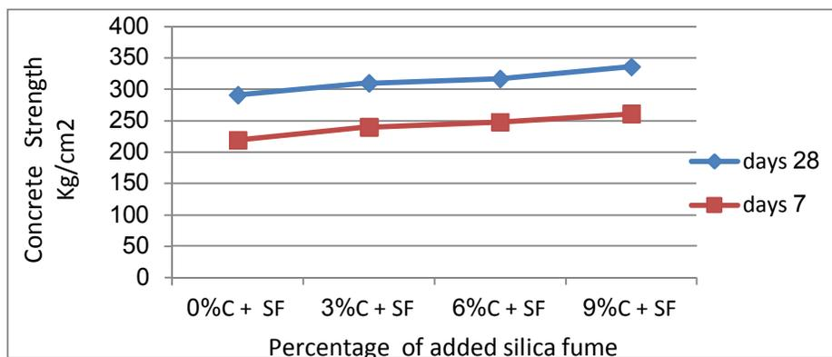
**Fig (1) Concrete strength Versus Percentage of added Silica Fume**
