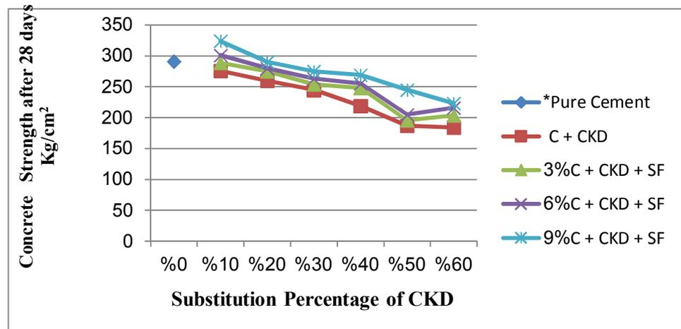
Fig(3) Concrete strength 28 days Versus Substitution percentage of CKD
