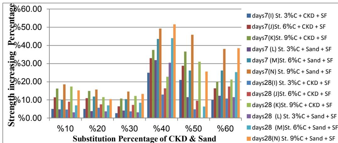
Fig (7) Percentage of Increasing Strength for substitution CKD, Sand and Silica Fume
