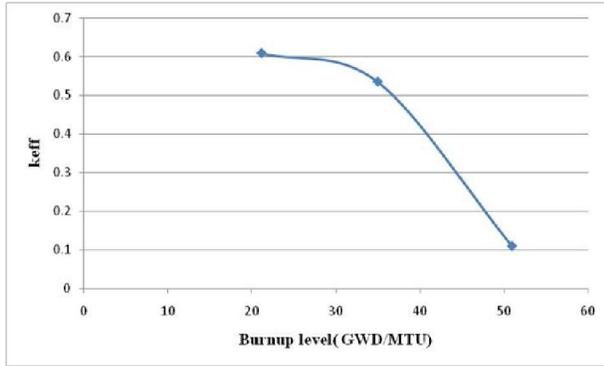
**Fig.10 k<sub>eff</sub> versus Burn-up level when assembly pitch = 0.0 cm**
