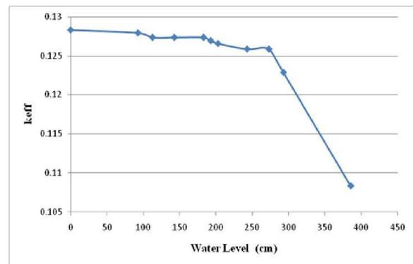
**Fig.9.  $k_{eff}$  versus Water level (cm) at BU= 64 GWD/MTU**
