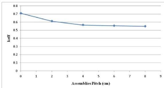
**Fig 4.  $k_{eff}$  versus Assembly Pitch (cm) with  $B_4C$  absorber**
