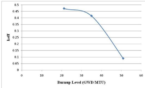
**Fig.11. k<sub>eff</sub> versus Burn-up level when Assembly pitch = 8.0 cm**
