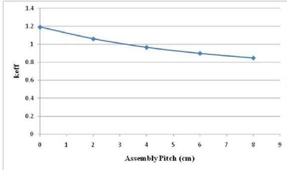
**Fig 3,  $k_{eff}$  versus Assembly pitch (cm) at no absorber**
