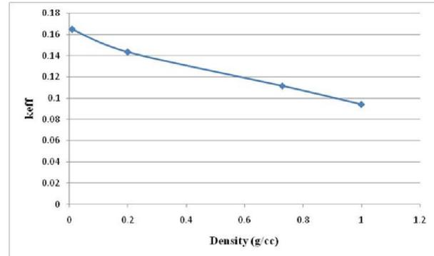
**Fig.13. k<sub>eff</sub> versus Water density, BU=51.967GWD/MTU at B<sub>4</sub>C absorber total volume, enrichment = 5% and assembly pitch =0.0 cm**
