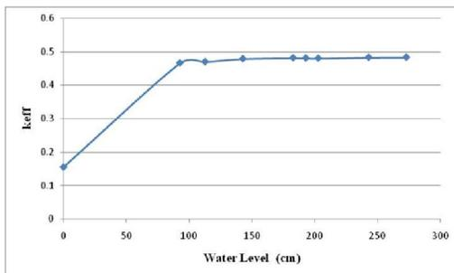
**Fig.7  $k_{eff}$  versus of Water level (cm) at BU= 21.17215GWD/MTU, pitch=0.0cm**
