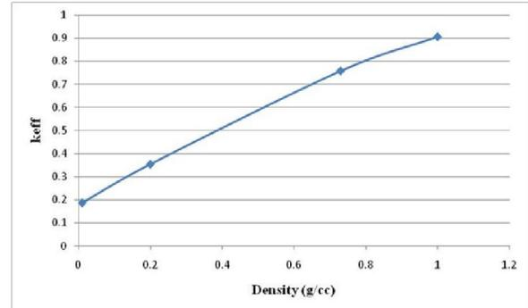
**Fig.12. k<sub>eff</sub> versus Water density, Fresh fuel, B<sub>4</sub>C absorber total volume when assembly pitch = 0.0 cm and enrichment = 5%.**
