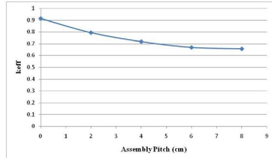
**Fig 5.  $k_{eff}$  versus Assembly pitch (cm) with Ag-In-Cd absorber.**
