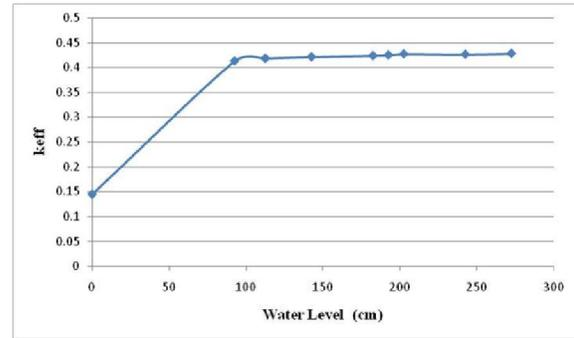
**Fig.8.  $k_{eff}$  versus Water level (cm) at BU= 35.030 GWD/MTU, pitch=0.0cm**
