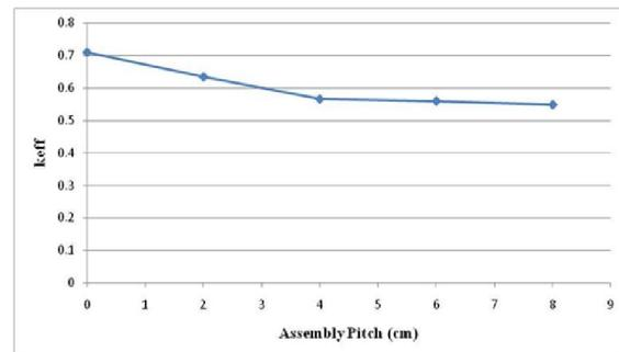
**Fig 6.  $k_{eff}$  versus Assembly pitch (cm) at BU= 56.5874 GWD/MTU**
