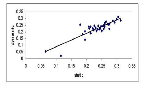
Diagram 3- correlation between Dynamic Contact Area A.I and Static Contact Area A.I data (r= 0.87)
