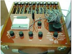
Figure 4. Daylighting factor meter
