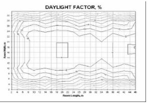
Figure 5. DF contour lines as measured in the simulation model of the hall and location of measured points
