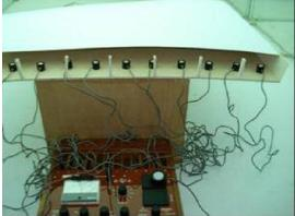
Figure 3. The model and daylighting factor meter
