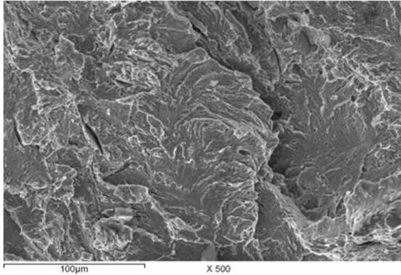
**Fig. 14 SEM observation of the fracture surface of cold cracked specimen at HAZ**
