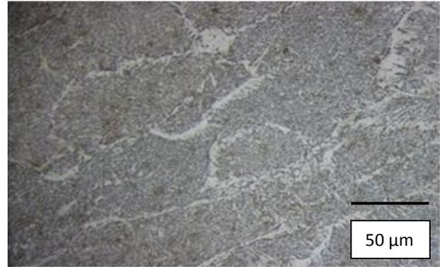
**Fig. 7** Microstructure of the weld metal using AWS A5.1 E7018 electrode
