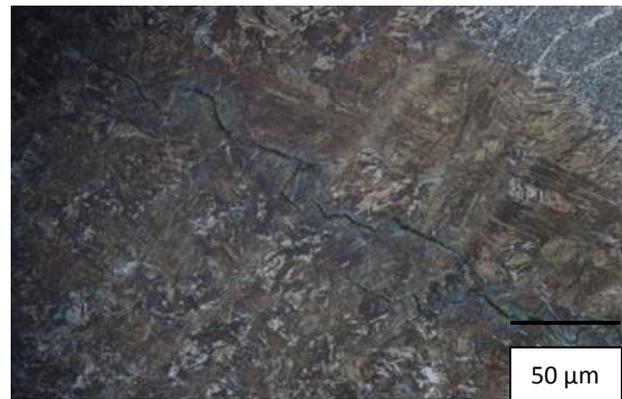
**Fig. 9** Microstructure at the cracked HAZ
