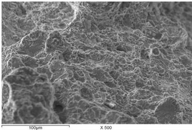
**Fig. 16 SEM observation of the fracture surface of cold cracked specimen at the weld metal**
