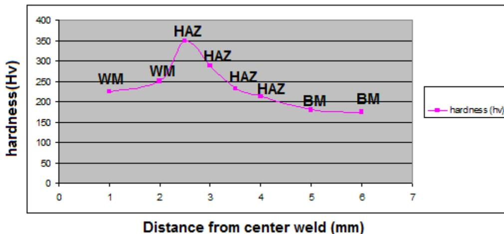
Fig. 13 Hardness distributions along weld metal, HAZ and base metal using E7018 electrode and applying a heat input of 1.34 kJ/mm without preheating
