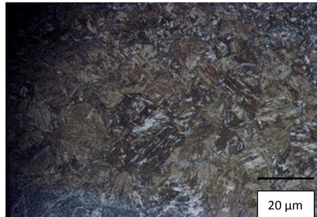
**Fig. 8** microstructure at the heat affected zone (HAZ)
