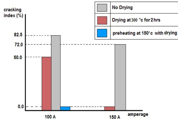
**Fig. 5** Effect of heat input on cracking index at different electrode conditions, welding current and preheating temperature
