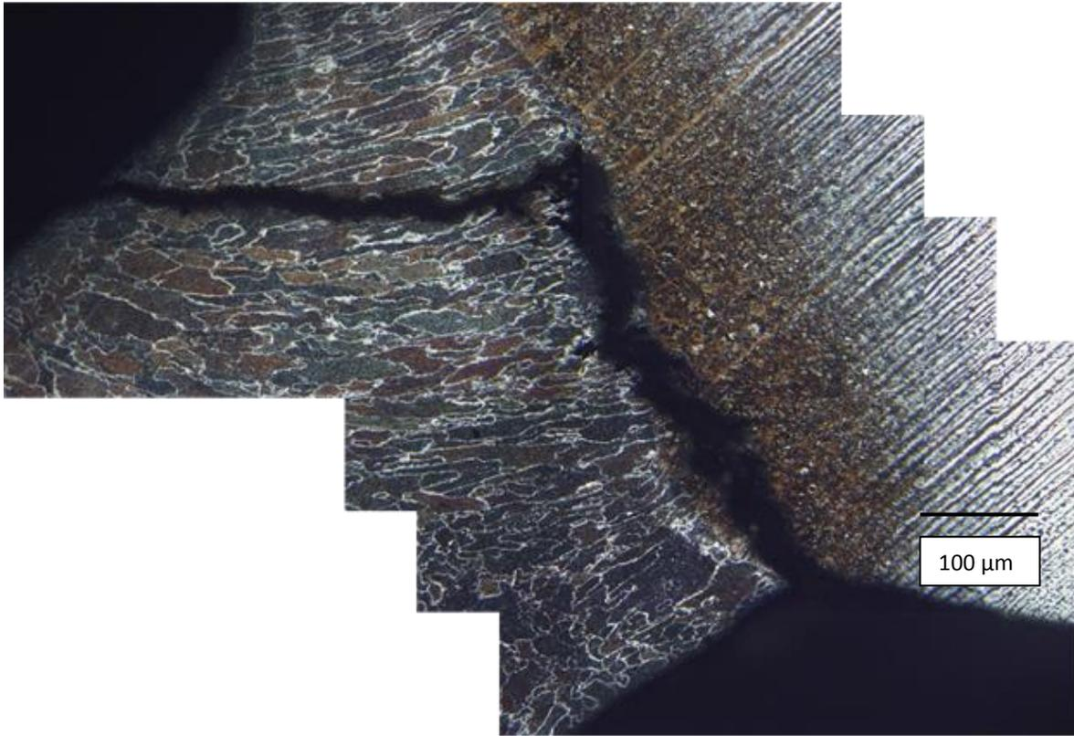
**Fig. 10** Microstructure at the cracked specimen where crack started at the root of the HAZ and propagated through HAZ and weld metal and finally terminated at the surface of weld metal.
