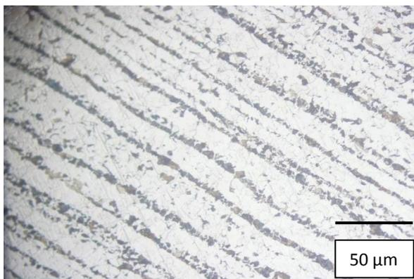
Fig. 1 Microstructure of ASTM A516 Gr 70 steel
