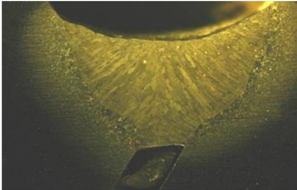
**Fig. 6** Macrostructure of the cross section of the test welded using a welding current of 150A with electrode dried at 300 °C for 2 hours and without preheating
