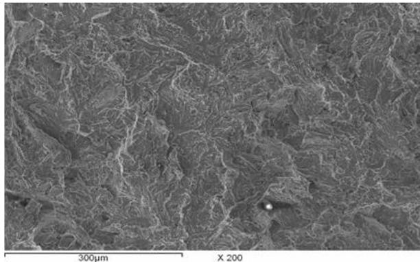
**Fig. 15 SEM observation of the fracture surface of cold cracked specimen at the transition between the weld metal and HAZ**
