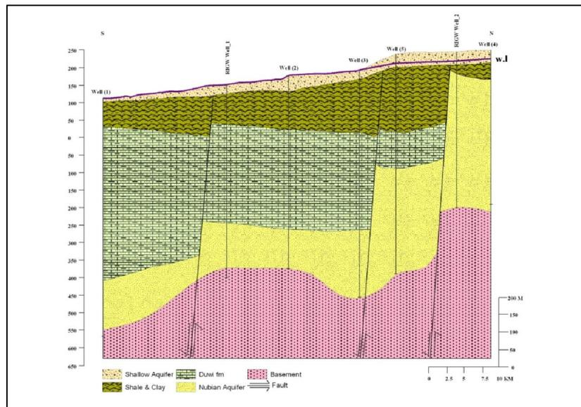
**Figure 2. Aquifer configuration of Wadi Qena**
