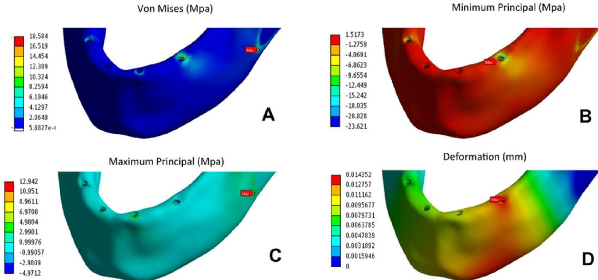
Fig. 4: Values of equivalent stresses, maximum and minimum principal stresses in MPa and deformation in mm for the cortical bone
