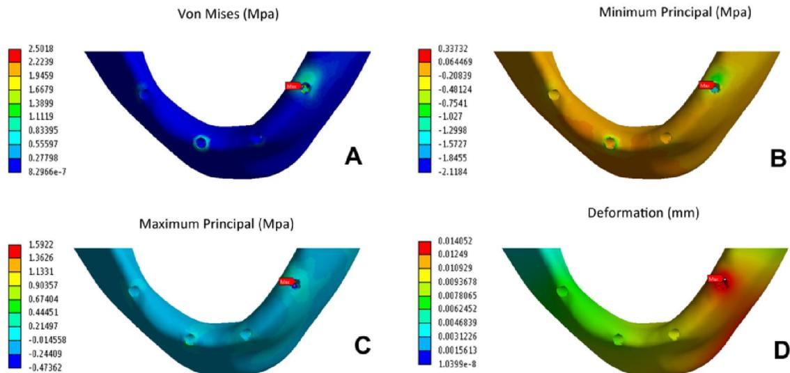
Fig. 5: Values of equivalent stresses, maximum and minimum principal stresses in MPa and deformation in mm for the trabecular bone
