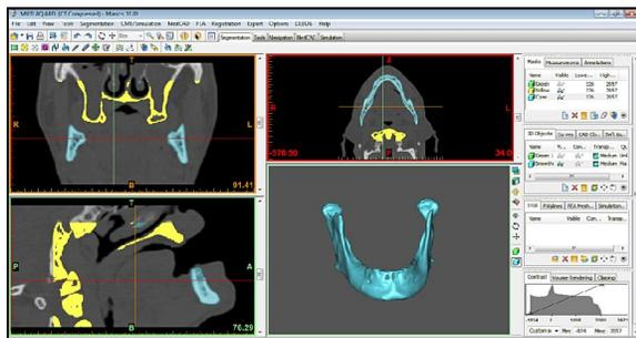
Fig. 1: Dicom images processed in Mimics software and converted both bone types to 3D STL file.
