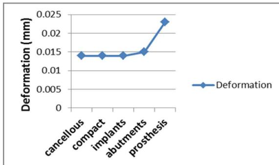
Fig. 10: Values of deformation in mm for bone, implants, abutments and the prosthesis.
