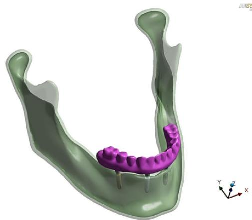
Fig. 2: The full design assembly imported to design modeler module of the finite element software.
