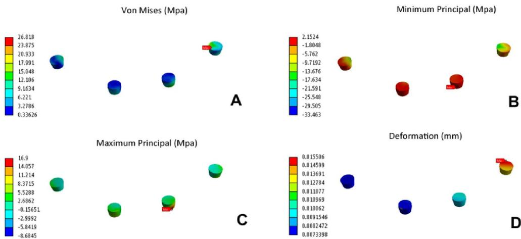
Fig. 7: Values of equivalent stresses, maximum and minimum principal stresses in MPa and deformation in mm for the abutments.
