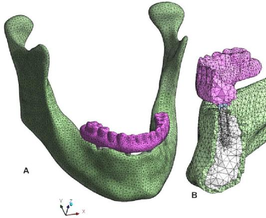
Fig. 3: Meshing of the model assembly using tetrahedron element type, A. A representative cross-section at molar areas showing elements in 3D seen in B.
