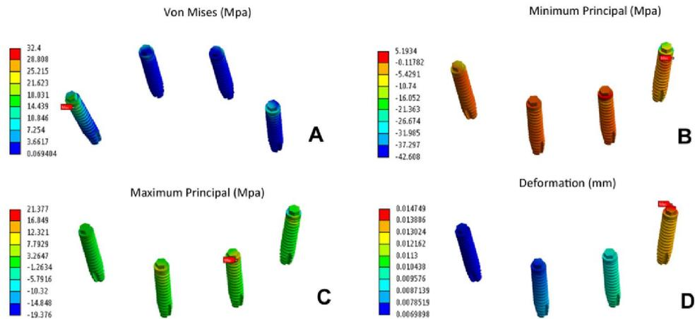
Fig. 6: Values of equivalent stresses, maximum and minimum principal stresses in MPa and deformation in mm for implants.
