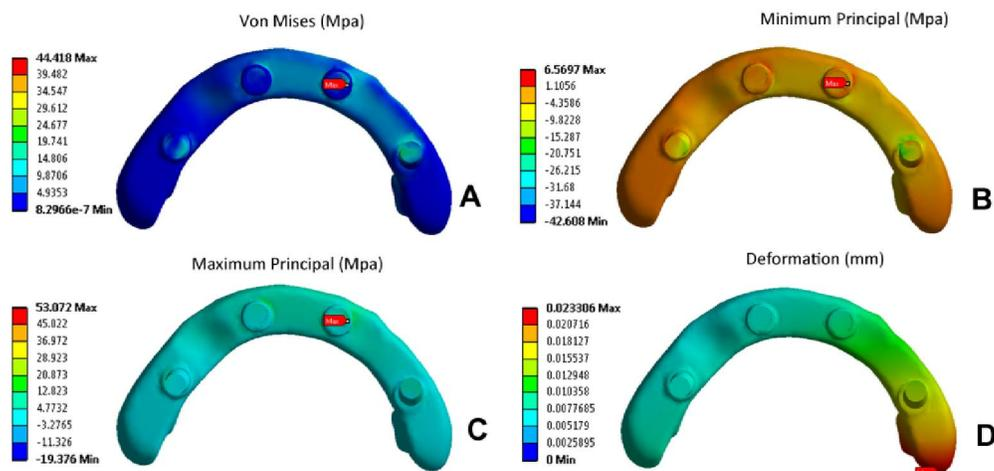
Fig. 8: Values of equivalent stresses, maximum and minimum principal stresses in MPa and deformation in mm for the prosthesis.
