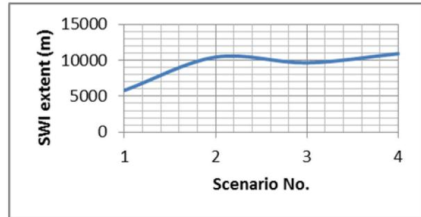
**Figure (10): In-land Seawater Intrusion for all scenarios at Ain Zara section.**
