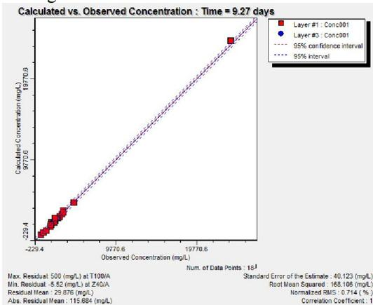
**Fig.(9) Steady state calibration results (TDS)**
