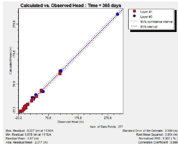
**Figure (8): Steady state calibration results (head)**
