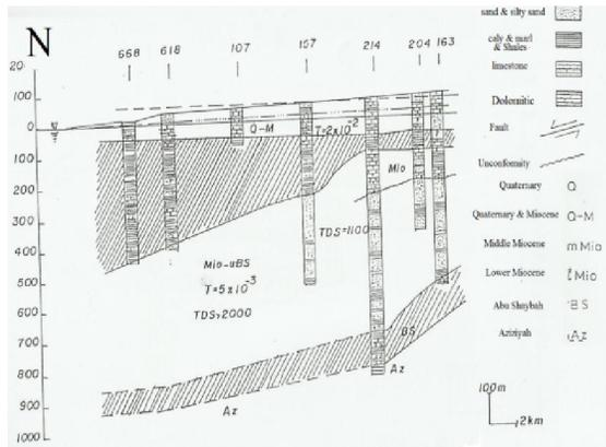
**Fig.3: Tripoli hydrogeological section (Kruseman and Floegel, 1978)**
