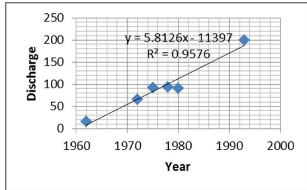
**Figure (6): interpolation of abstraction rate from 1962 to 1993 (municipal).**
