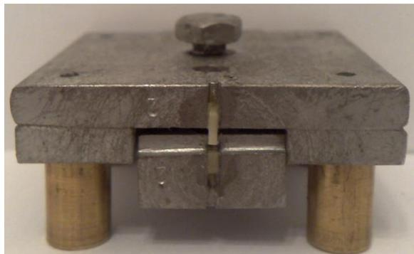
Figure 2. Attachment jig with a glued beam specimen immediately after its tensile straining to failure.
