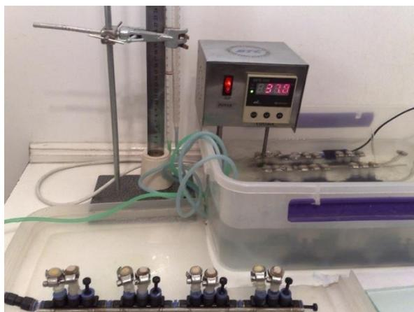
Figure 1. The water bath container connected to the perfusion system and the temperature controlling unit is showing the water temperature. A row of teeth was removed from the container for adhesive application and composite buildup.
