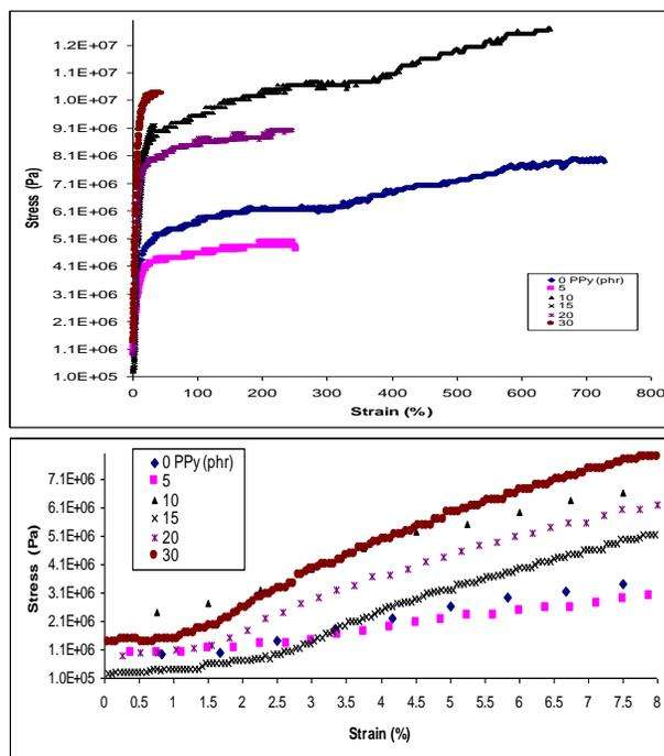
**Figure (2): The nominal stress –strain curves for the composite up to 30 phr of PPy.**
