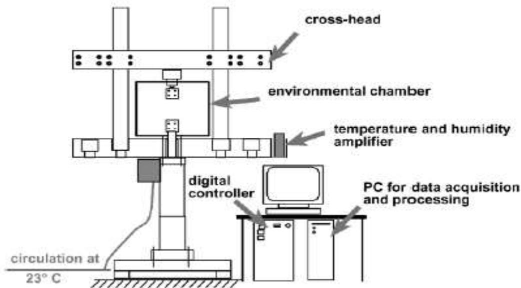
**Figure (1): Shows the system used in measuring mechanical properties**
