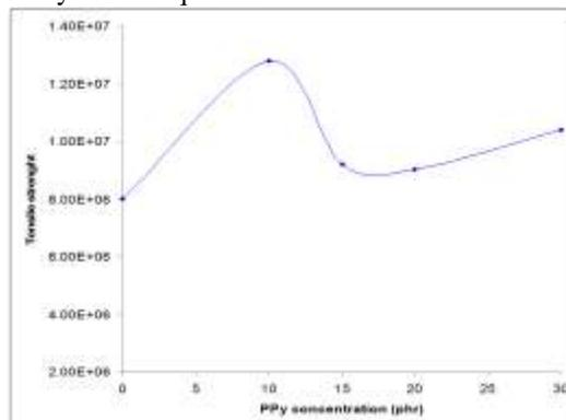
**Figure (4): The tensile strength for all samples of PPy/EVA composites with sample concentration.**
