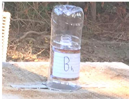
Fig. 2: Magnified view for insect collection bottle
